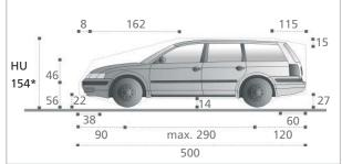
max. car width 190cm, max. load per platform 2000kg, max. load of wheel 500kg
